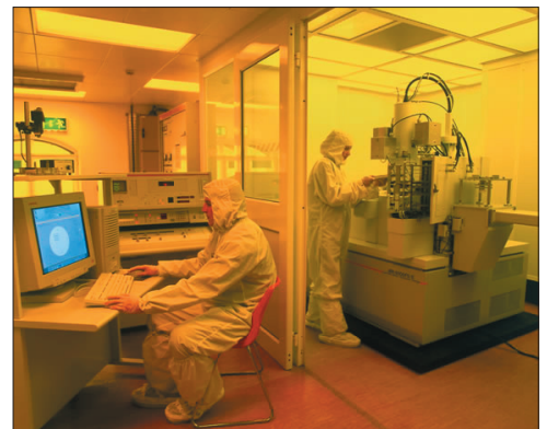
Above: Jeol 6000FS Electron beam lithography system
