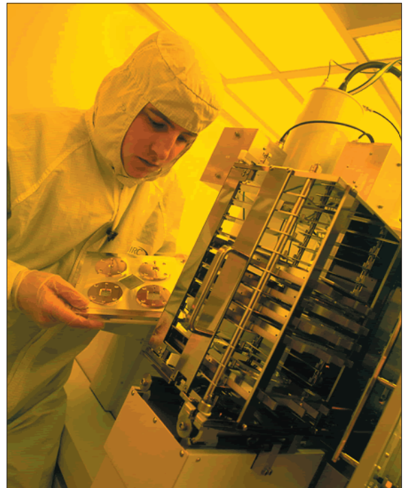
Above: Loading the substrate holder magazine on the Jeol 6000FS
