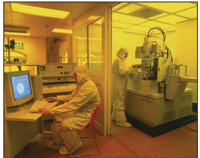
Above: JOEL 6000F3 e-beam equipment in use in the clean room
