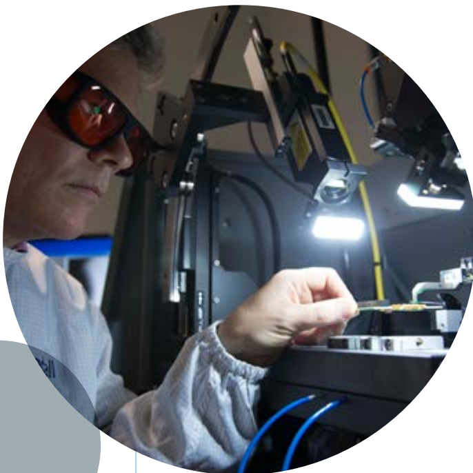
Dr Peter O'Brien using a laser welding machine in Tyndall's photonics packaging lab to actively align an optical fibre with photonic integrated circuits under sub-micrometre tolerance.
