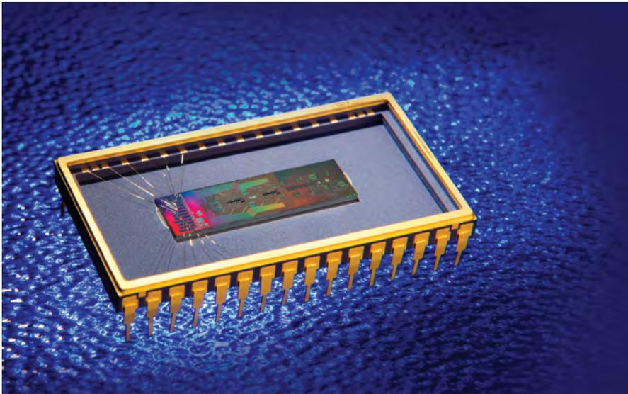
Packaged CMOS sensor silicon chips demonstrated a next-generation CMOS diagnostics platform developed under the Enterprise Ireland Innovation Partnership Programme, in conjunction with Altratech.
