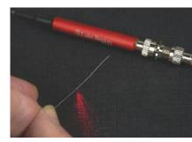
Photonic sensor technology in medical guidewire.
