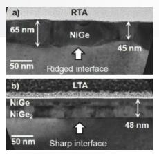
Representative Cross-Sectional Transmission Electron Microscopy Images of Nige Layers Formed By **(a)** 350°C Rapid Thermal Anneal (RTA) and **(b)** Laser Thermal Anneal (LTA) With Energy Density of 0.45 J/CM<sup>2</sup>.
