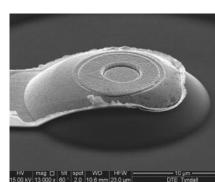
A single 16µm diameter DUV microLED.
