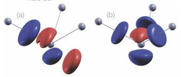
Changes in electron density induced by optical excitation in bismuth for two different directions of light polarization. By choosing the light polarization, different types of atomic motion can be induced.
