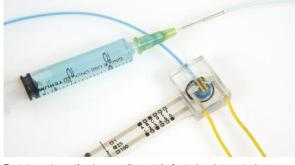
Prototype 'smart' microneedle patch featuring integrated pressure and impedance sensors for real-time delivery system performance monitoring and control.
