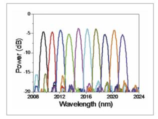
Two micron wavelength optoelectronic device results.
