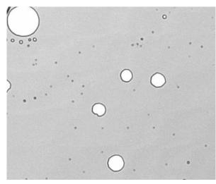
Acoustic image of bonded Si-to-Si wafer structure showing voided areas.
