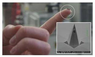
Hollow microneedles customised to deliver local anaesthetic during dental procedures.
