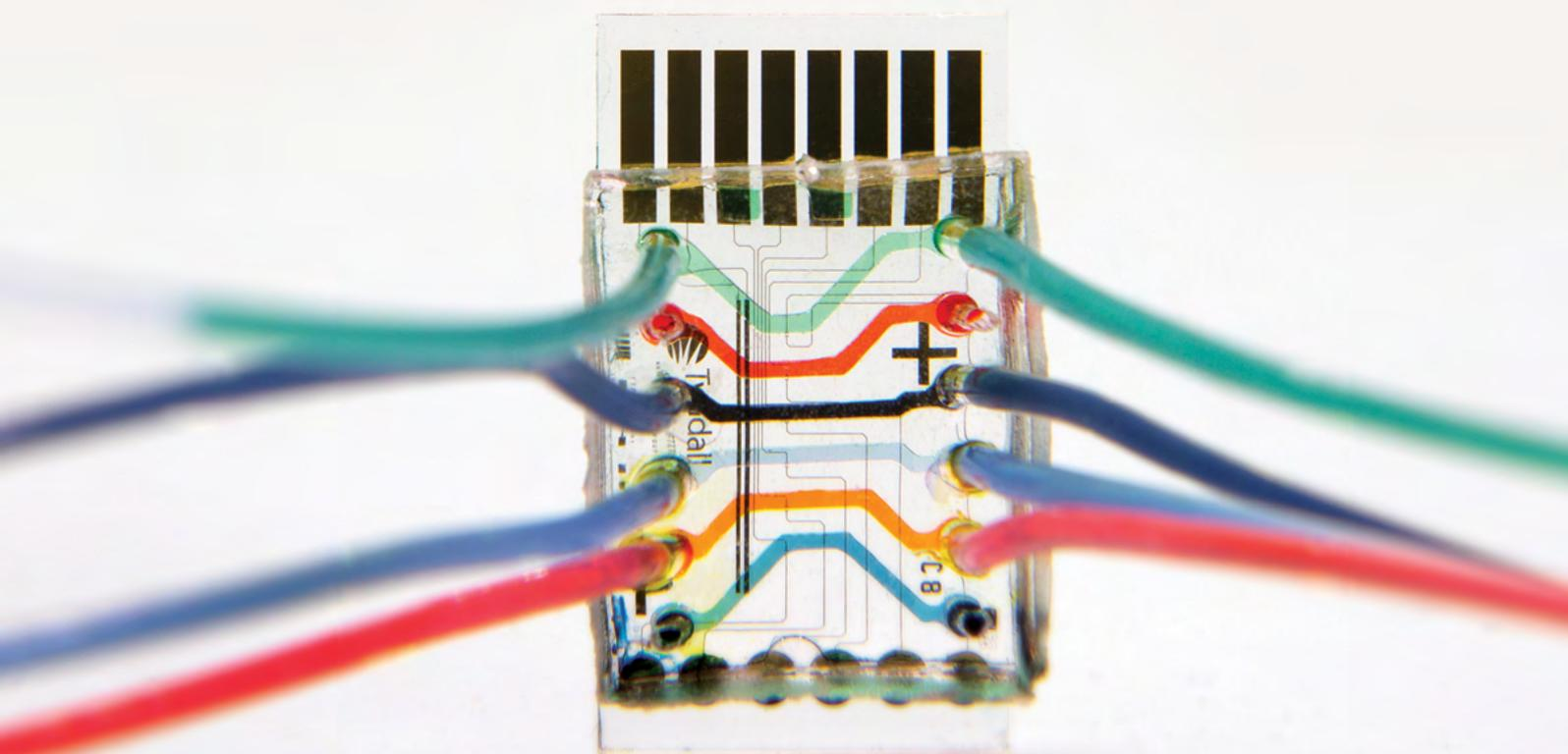
Integrated nanosensor chip coupled with a microfluidic sampling device used to deliver rapid disease detection in cattle.
