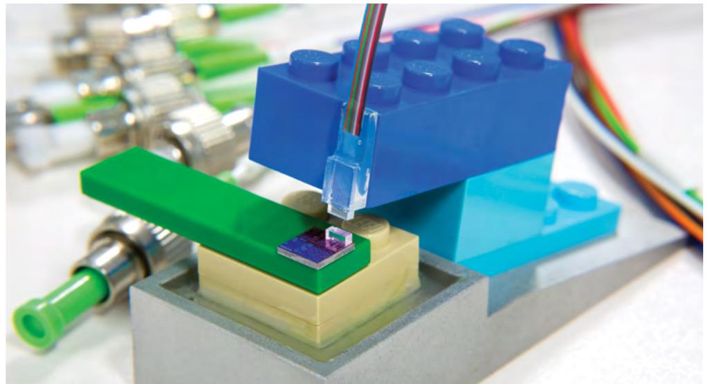
Pluggable multi-channel single mode optical connector to silicon photonic integrated circuit.
