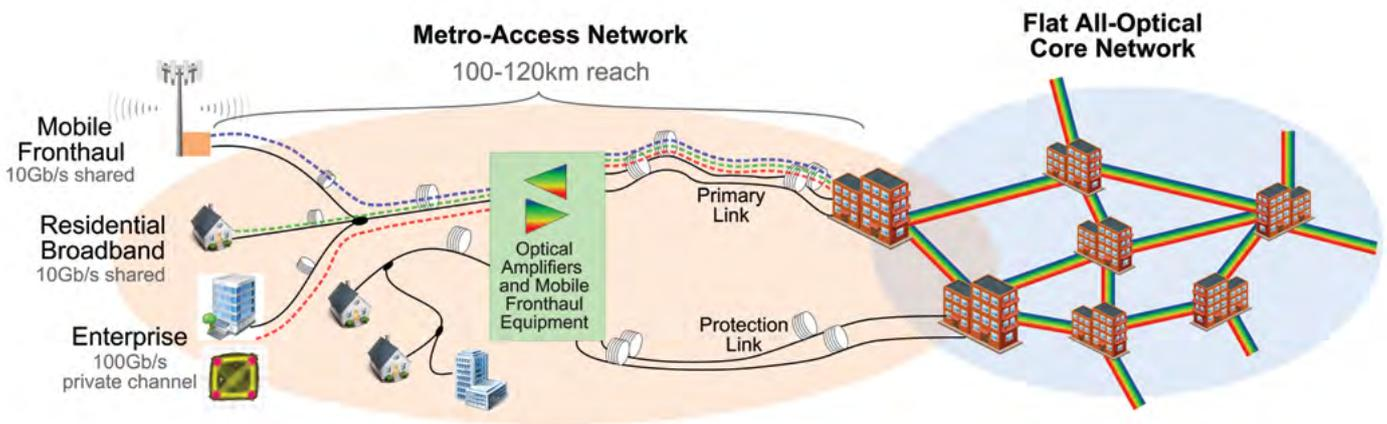
A collaboration between Tyndall’s Photonic Systems Group, Trinity College Dublin and industry partners Nokia Bell Labs and Polatis has developed the world’s most advanced demonstration of a new, highly scalable network architecture based on long reach fibre access networks.
