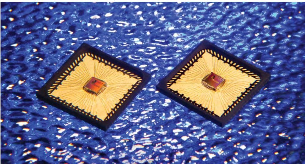
Packaged CMOS chips, consisting of an Ultra-low Power SAR ADC to enable next-generation deployed IoT Sensor nodes, developed in conjunction with S3 Group under the Enterprise Ireland Innovation Partnership Programme.
