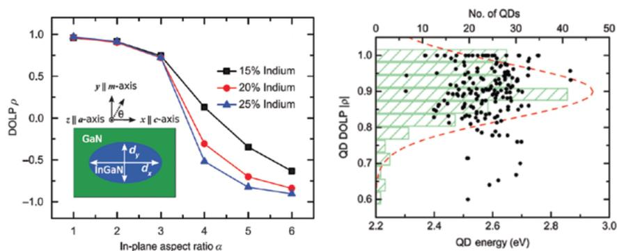
Polarised single-photon sources are essential for applications in quantum information systems, such as quantum key distribution. To develop these non-classical light sources, semiconductor nanostructures, such as quantum dots, have been of strong scientific interest. Here, nitride-based materials have attracted considerable attention since their fundamental properties put room temperature single-photon emission within reach.
