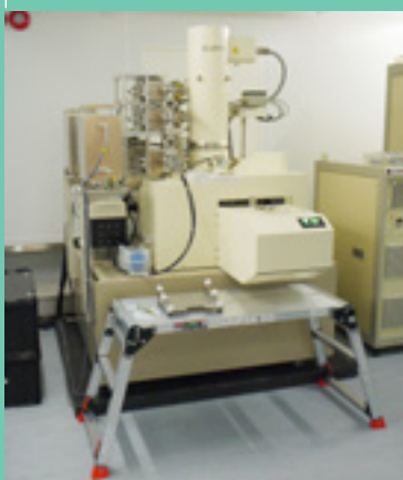
Elionix e-beam – 6 nm on 200 mm wafers
